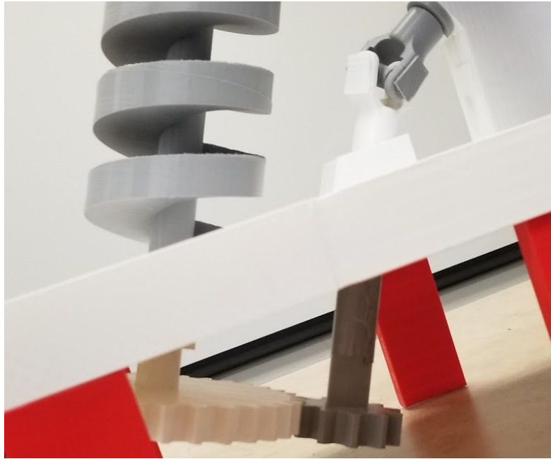
Figure 4: Connecting Rod to Archimedes Screw
