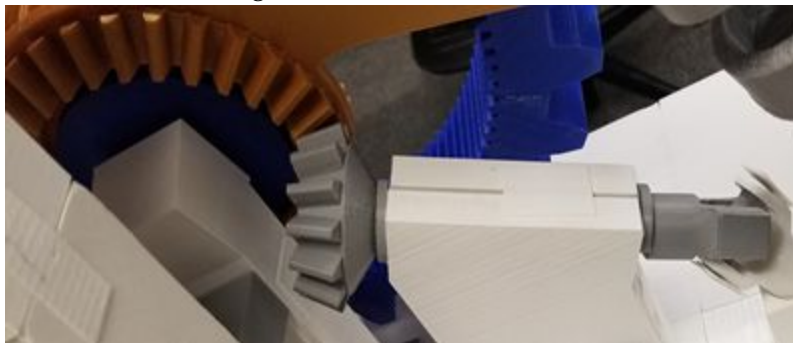
Figure 3: Bevel Gear on Back of Planet Gear Holder
